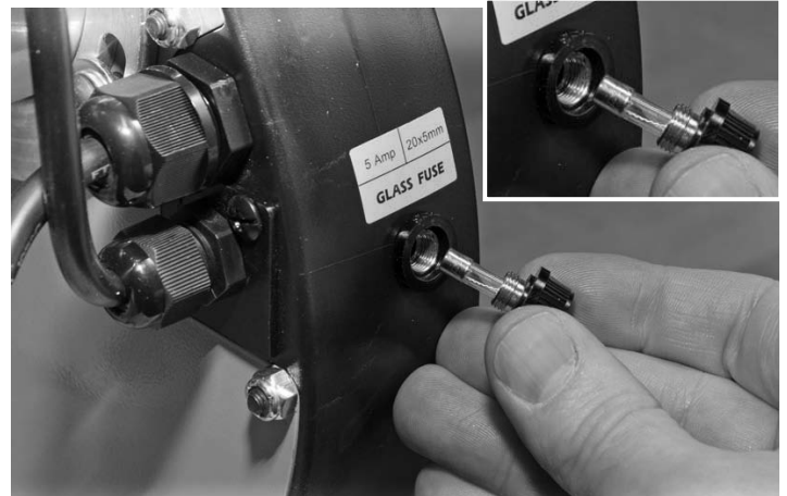
3. Insert a new 5 AMP fuse into the end cap holder.
