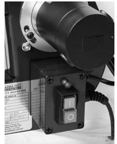
NVR power isolating switch
